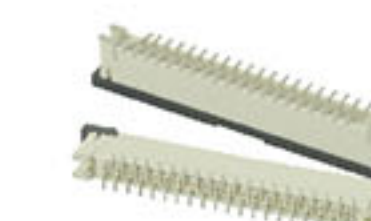
FPC, Vertical 312A-XXNAA-R 312A-XXRAA-R, Reverse Pitch: 0.5mm, H=5.95mm
