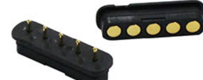
Pogo Pin, Waterproof Type 303C-C3018-25-05, w/o Cap 5 Pin PH 2.5mm, T/L 6.6mm, w/H 1.2mm
