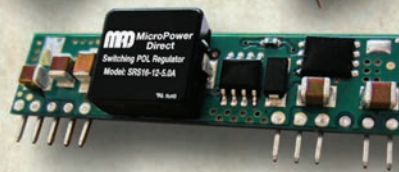
Switching POL Regulators
