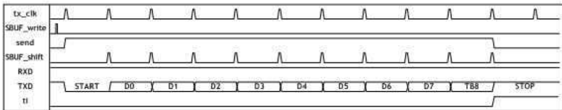
Figure 6.9 Timing Diagram for UART Transmission Mode2
