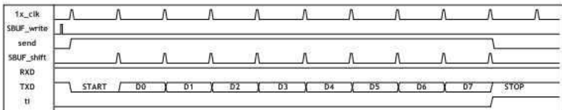
Figure 6.8 Timing Diagram for UART Transmission Mode1
